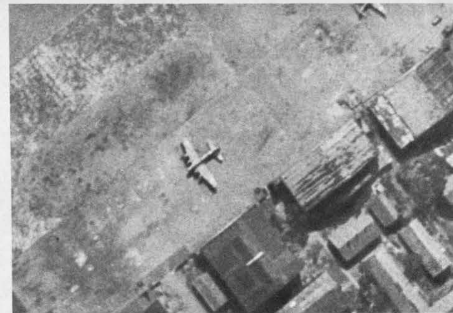
Four-engine Tachikawa Field 104 may be a transport or long-range bomber. Broad wing is set low or mid-low on round fuselage somewhat like that on two-engine Betty.
